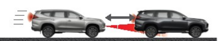
When the vehicle in front slows or stops, ACC slows or stops your vehicle.
