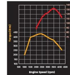
2.4-liter MIVEC Turbocharged DOHC DI-D High power (133kW/3500rpm)
