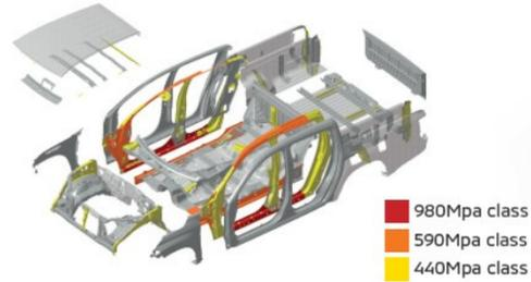
The body is extremely sturdy and lightweight due to the generous use of high tensile strength steel plates that also contribute to a high level of collision safety.
