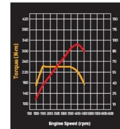
2.5-liter Intercooled Turbocharged DOHC DI-D (94kW/4000rpm)
