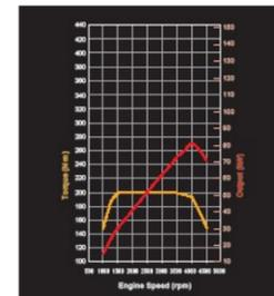
2.5-liter Turbocharged DOHC DI-D (81kW/4000rpm)
