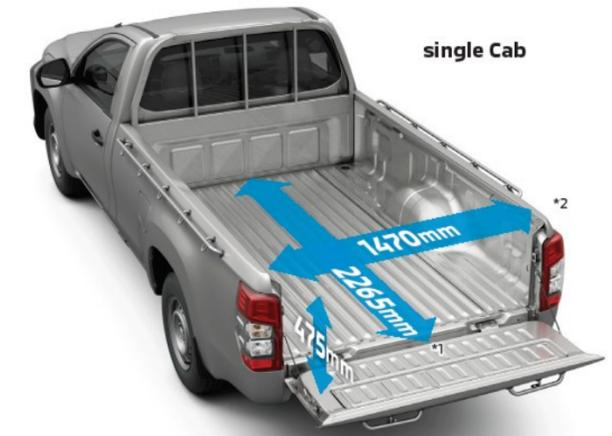
\*1: Measured from bottom of bed \*2: Measured from top edges
