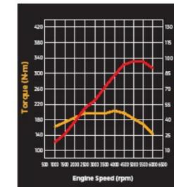
2.4-liter SOHC 16-valve MPI (97kW/5250rpm)
