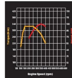
2.4-liter Intercooled Turbocharged DOHC DI-D (100kW/3500rpm)
