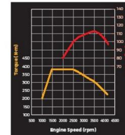
2.4-liter Intercooled Turbocharged DOHC DI-D Standard (113kW/3500rpm)
